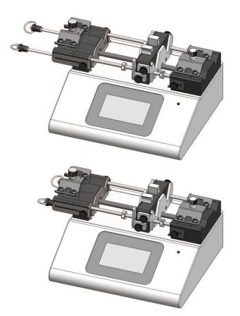
Large syringes can acheive full stroke length by repositioning the adjustable syringe holder.
